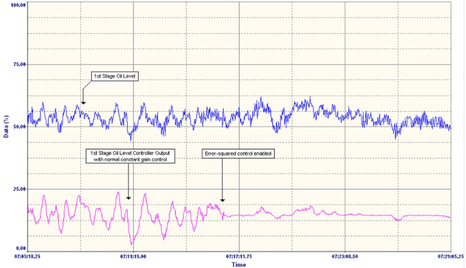
**Figure 1. Trend of a separator level controller before and after initiating error squared**
