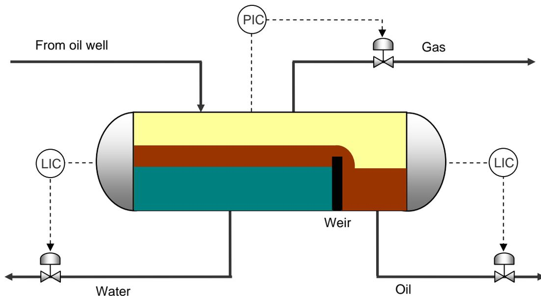
**Figure 3. Separator control loops**
