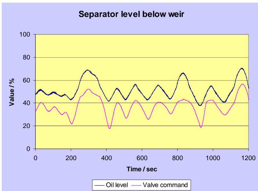
**Figure 4. Separator oil level and control valve output**
