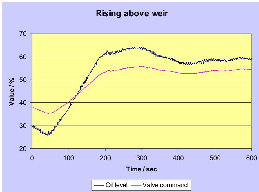
**Figure 5. Separator oil level rising above weir**
