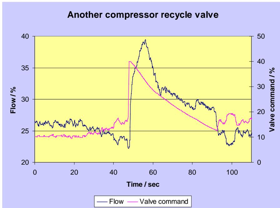
**Figure 11. Another valve not lifting smoothly off seat**
