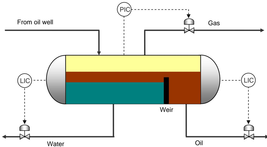
**Figure 6. Flooded weir operation**
