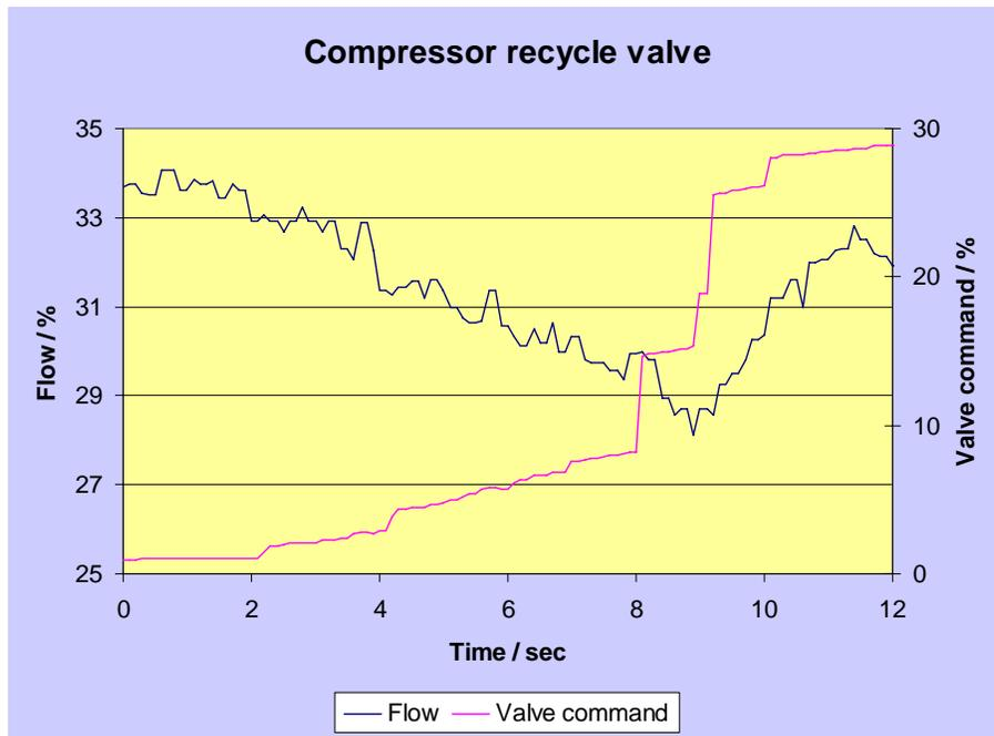
**Figure 10. Effects of valve not lifting from seat**
